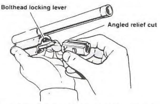
The angled relief cut on the bolt assembly will push the locking lever up.
